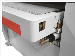
Pneumatic conveyor belt tracking
