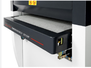
Over height material gate and emergency bump bar
