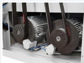
Pneumatic disc brakes for sanding heads
