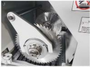
MRS340M1 with single moving blade and fixed saw blade
