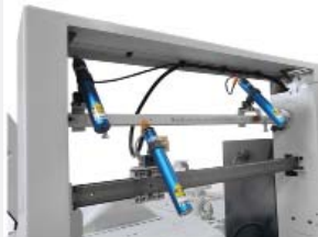
Projection laser for identifying the cutting line
