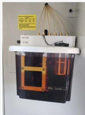
Automatic lubrication unit for the chain track assembly
