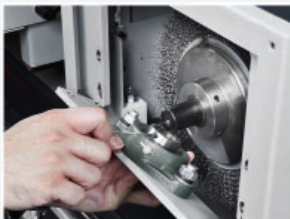
Outboard bearing to support the brushing spindle
