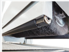
Spring loaded rubber hold down rollers before and after each brushing unit
