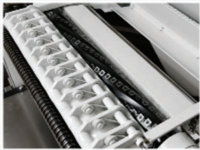
Spiral insert knife cutterhead
