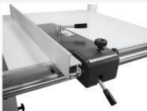
Precision rip fence with fine adjustment
